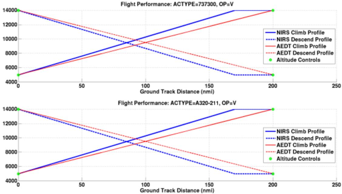
Figure E-6: Representative Overflight Profiles (Altitude in AFE)
