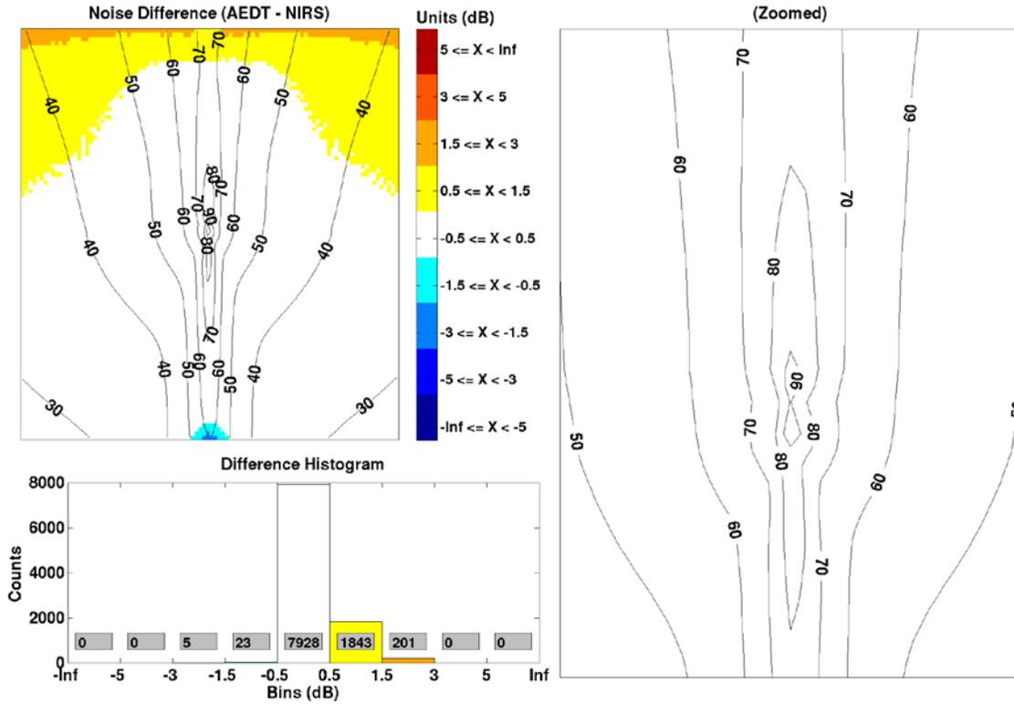
Figure 3-17: WEST (AEDT 2a-NIRS) SEL Noise Difference (Equal Grids)
