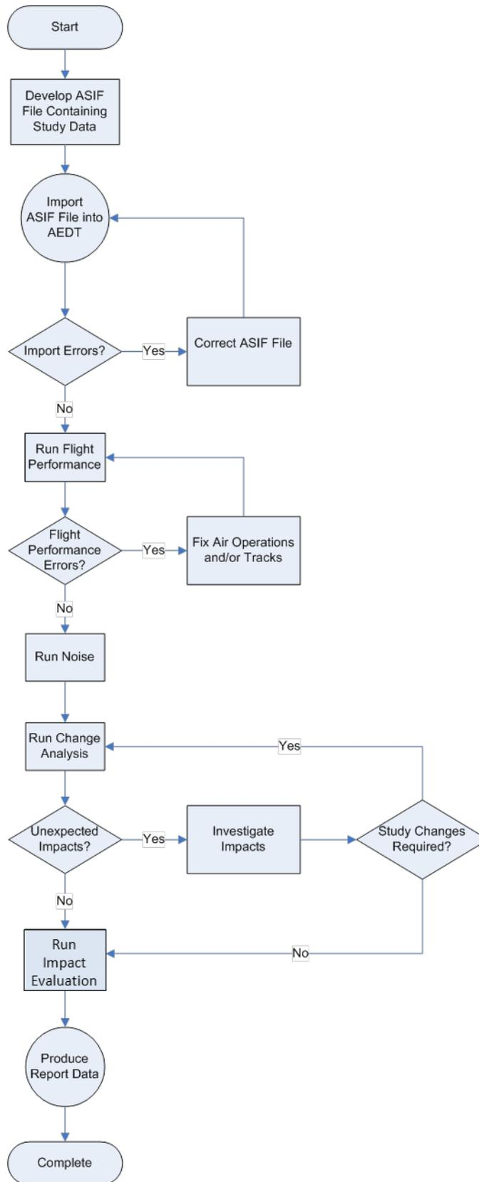
Figure B-0-1: Applicable Environmental Study Generic Workflow Diagram
