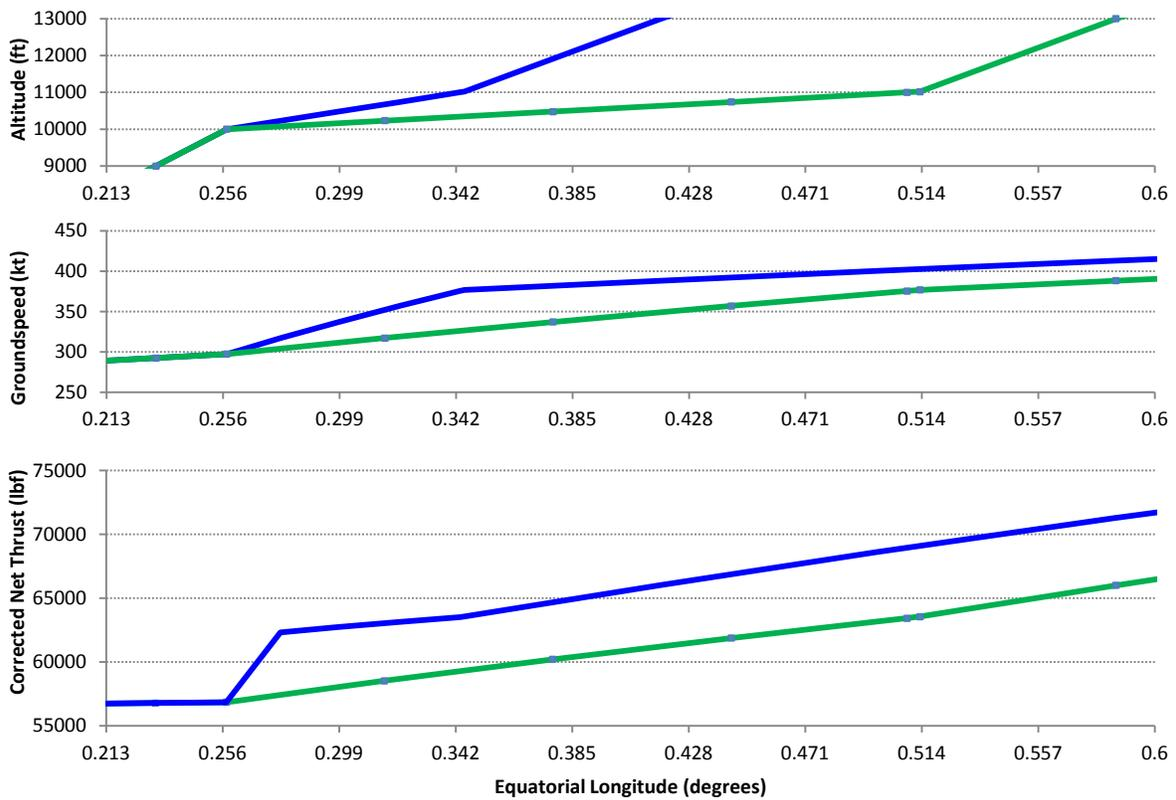
Figure 3–46: Transition from 1845/Doc. 29 to BADA – AEDT 2a (Green) vs. AEDT Development Versions (Blue)
