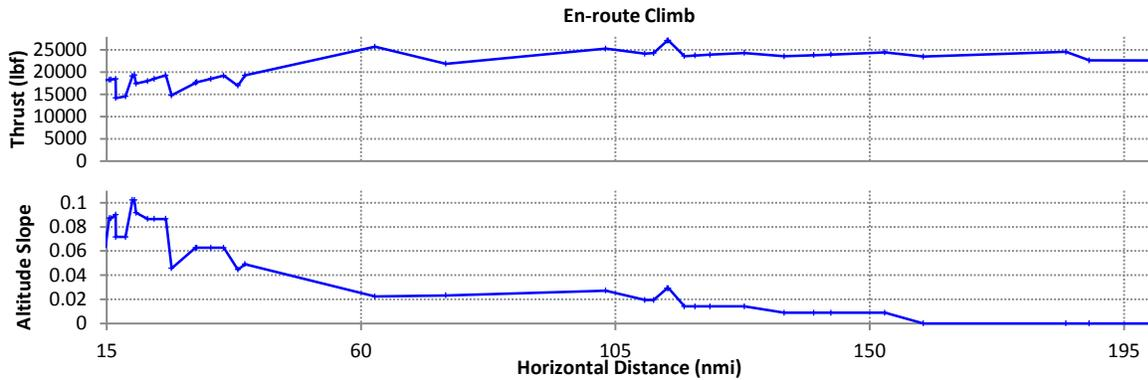
**Figure 3–39: Thrust and altitude slope for the en-route climb portion of a flight from KSAN to KJFK, based on smoothed and filtered data**
