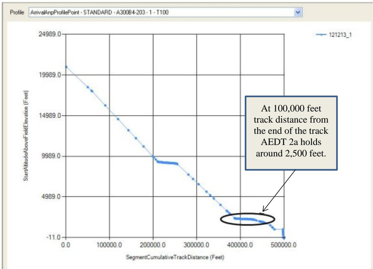
Figure 4–12: AEDT 2a Arrival Profile for A300B4-203 on Track T100
