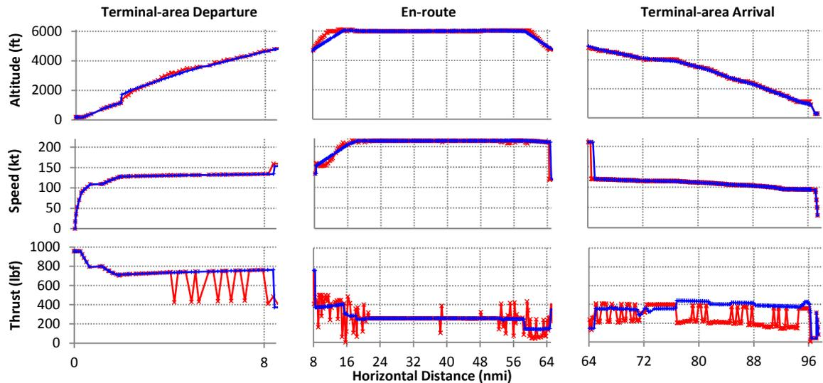
**Figure 3–40: Altitude above mean sea level, groundspeed, and corrected net thrust for the en-route portion of a flight from KRIC to KIAD, based on raw data (red) and on smoothed and filtered data (blue)**
