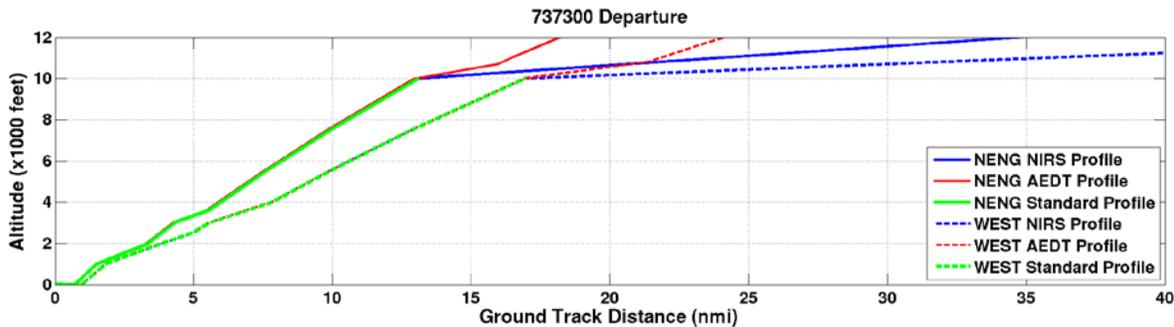
Figure 3–9: Environmental Parameters Test Departure Flight Performance, Altitude in AFE
