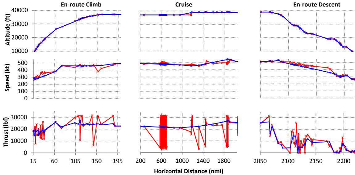
Figure 3–37: Altitude above mean sea level, groundspeed, and corrected net thrust for the en-route portion of a flight from KSAN to KJFK, based on raw data (red) and on smoothed and filtered data (blue)
