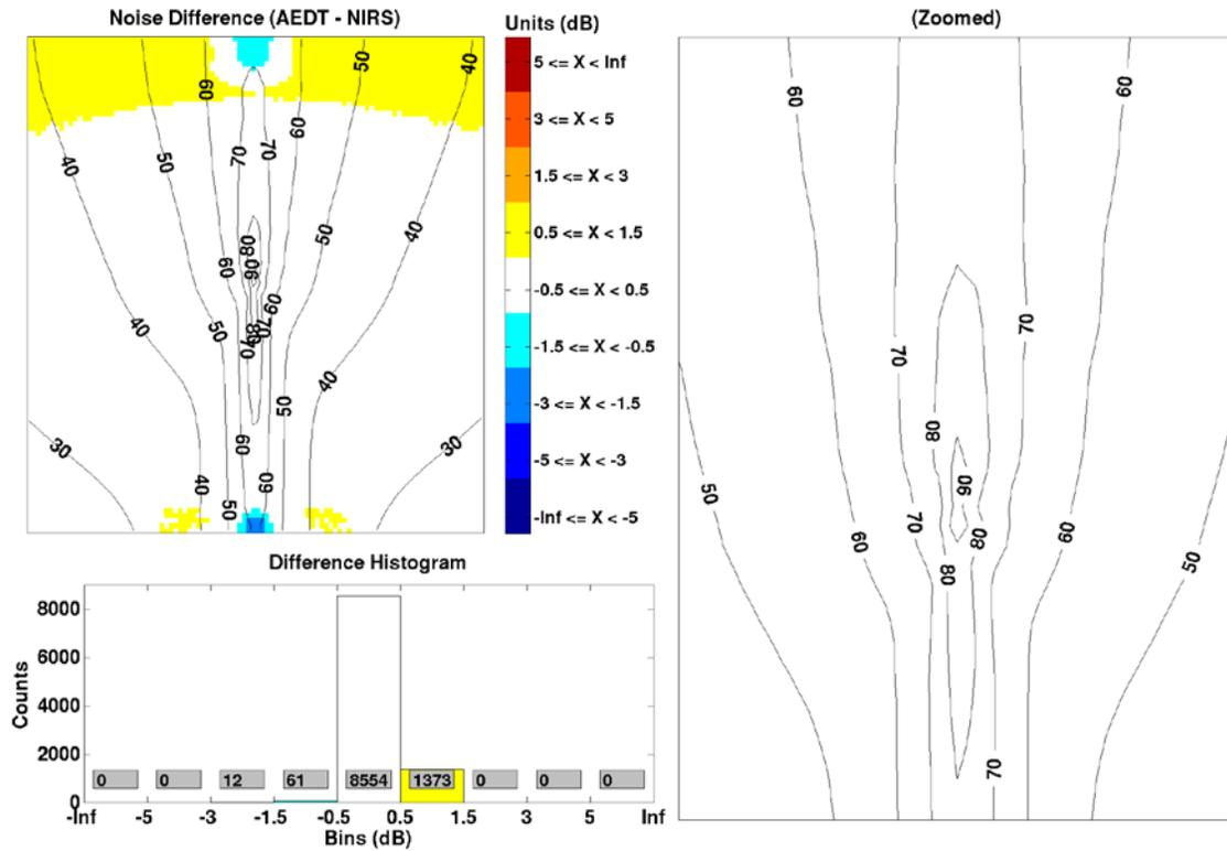
Figure 3-15: NENG (AEDT 2a-NIRS) SEL Noise Difference (Equal Grids)
