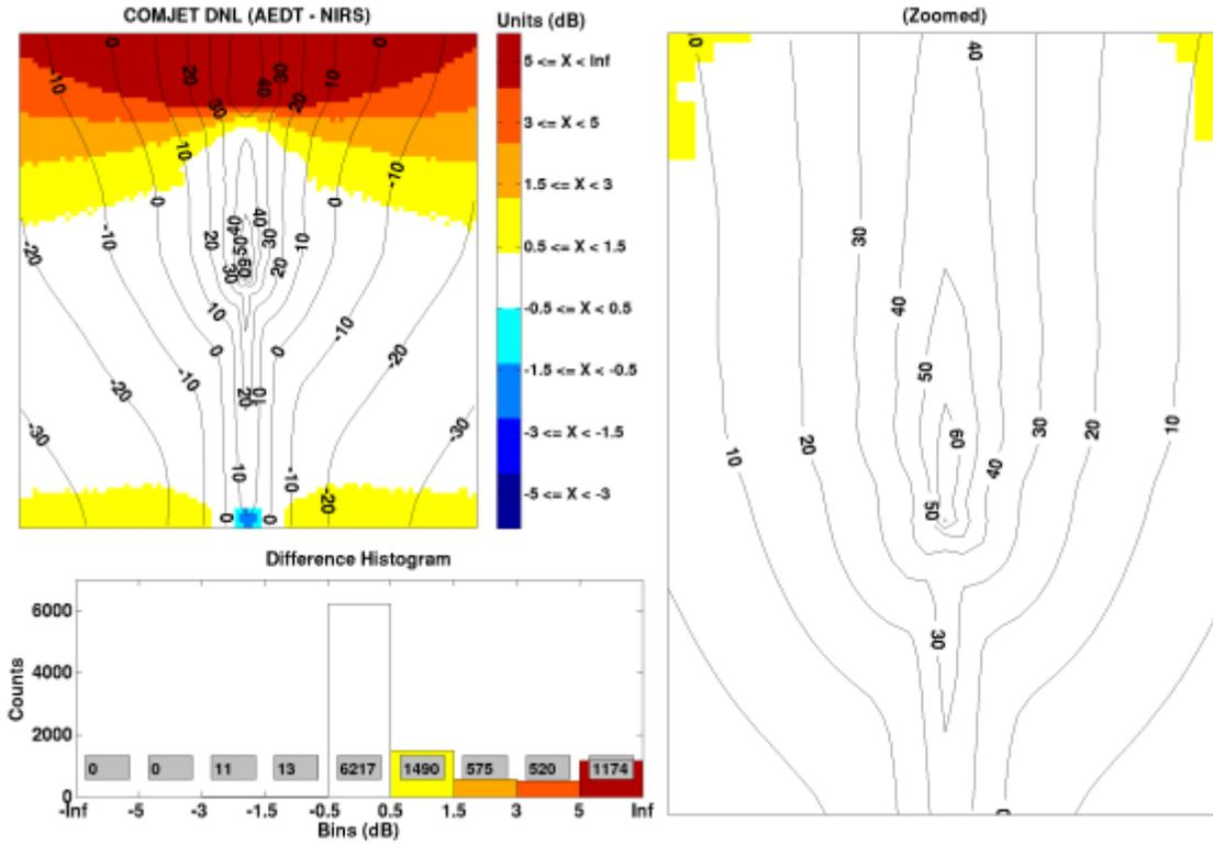
Figure D-7: COMJET DNL Noise Differences
