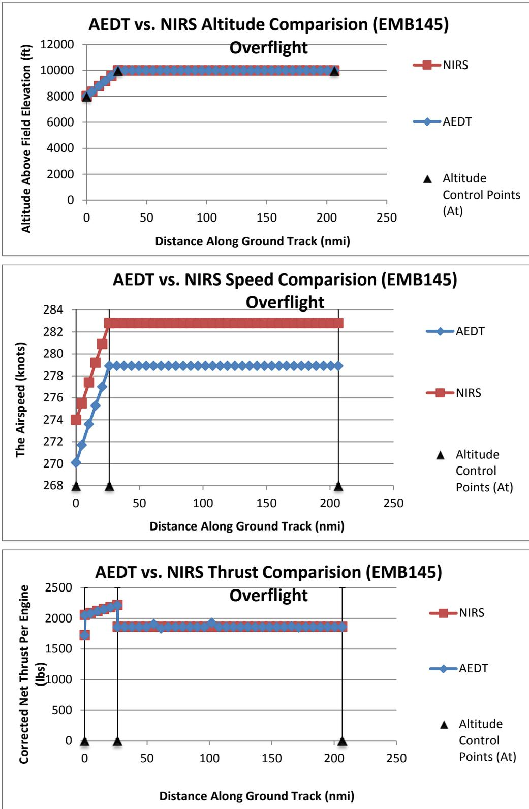
Figure A-8: EAST\_MED Overflight Comparison – EMB145
