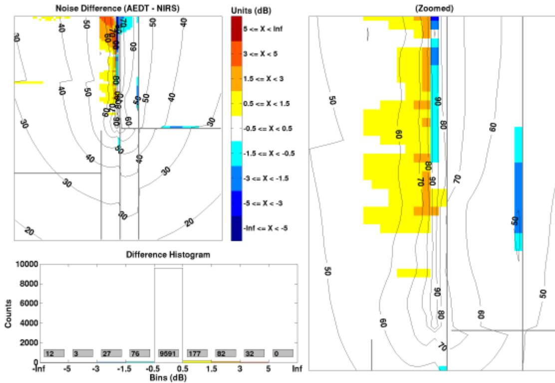
Figure 3-24: AEDT 2a- NIRS Straight Departure Differences with Terrain
