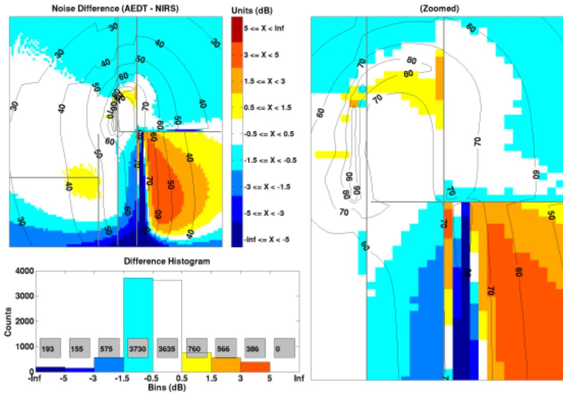
Figure 3-26: AEDT 2a- NIRS Curved Departure Differences with Terrain
