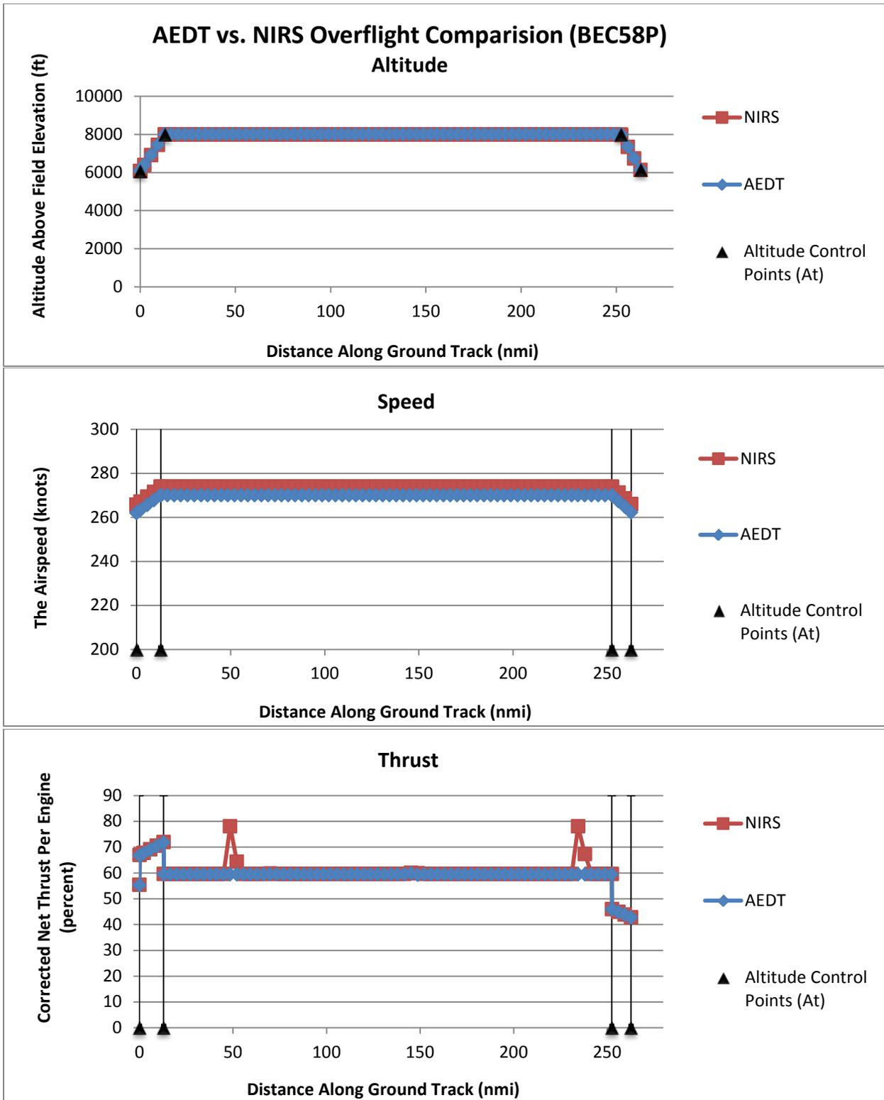
Figure 3-6: EAST\_MED Overflight Comparison – BEC58P
