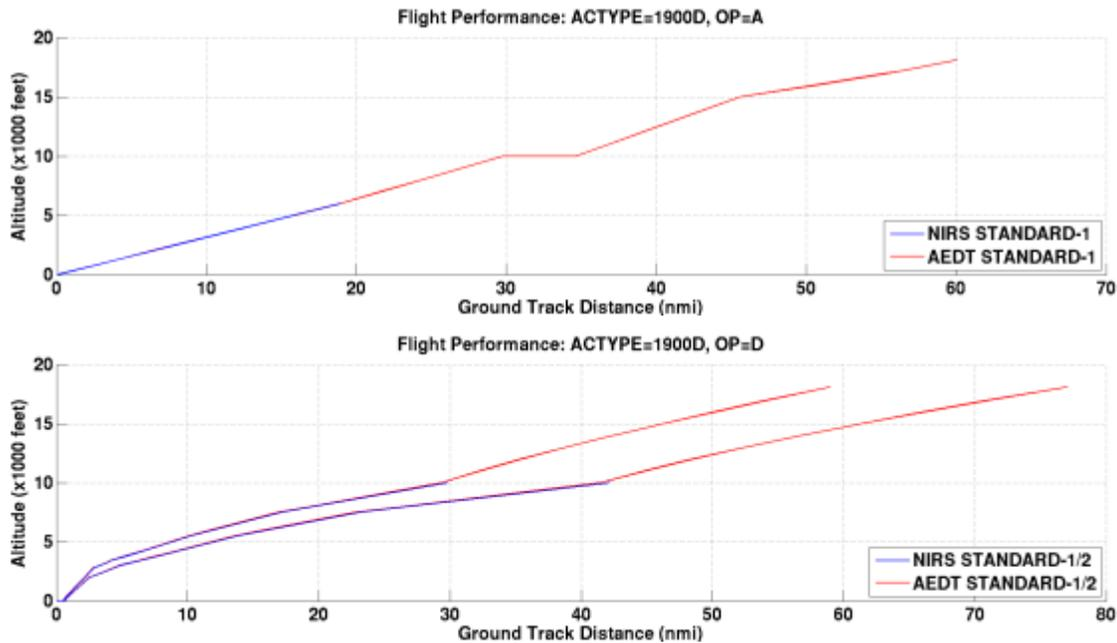
Figure E-2: 1900D Default Flight Performance (Altitude in AFE)
