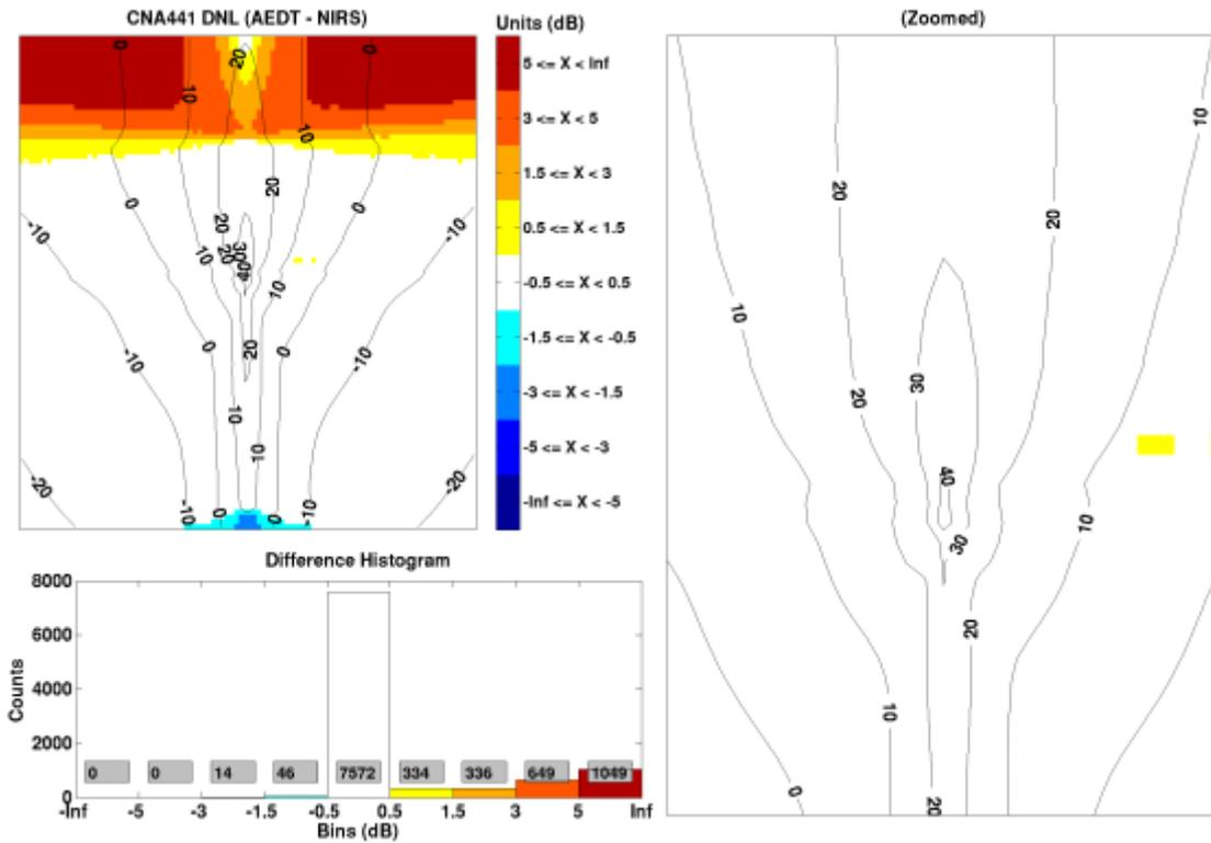
Figure D-6: CNA441 DNL Noise Differences
