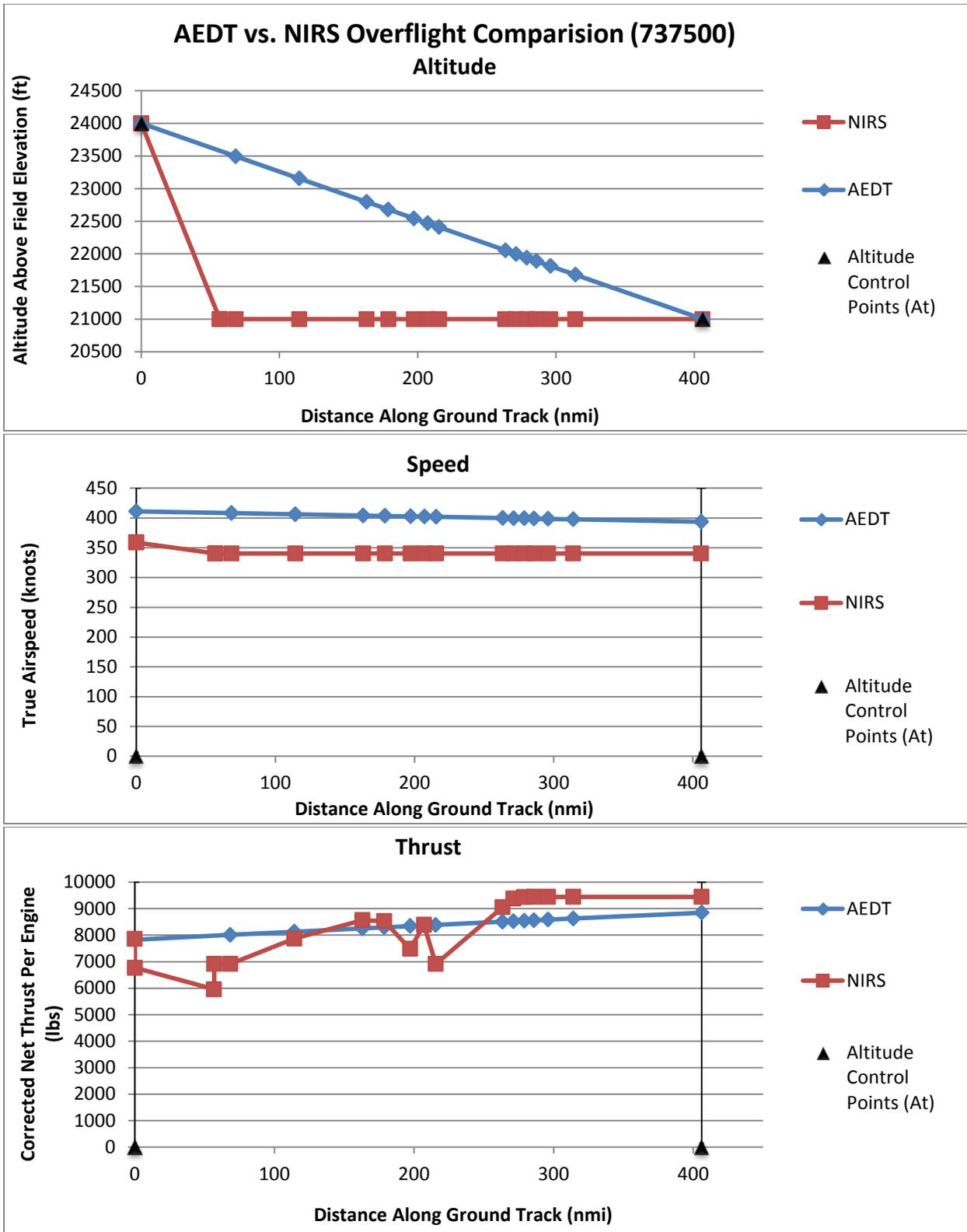
Figure 3-3: STUDY\_NIRS Overflight Comparison – 737500
