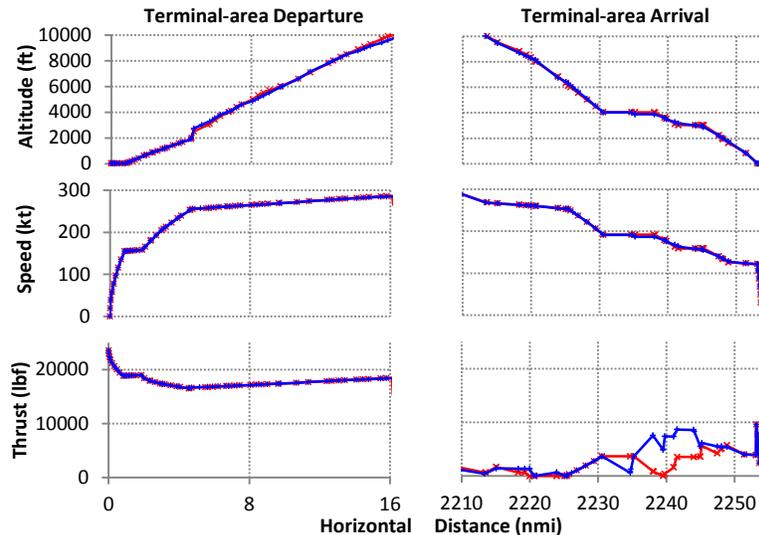
Figure 3–38: Altitude above mean sea level, groundspeed, and corrected net thrust for the terminal-area portions of a flight from KSAN to KJFK, based on raw data (red) and on smoothed and filtered data (blue)
