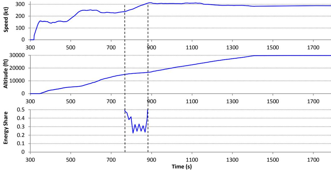
**Figure 3–47: The Effects of Increasing Energy Share During Accelerated Climbs**
