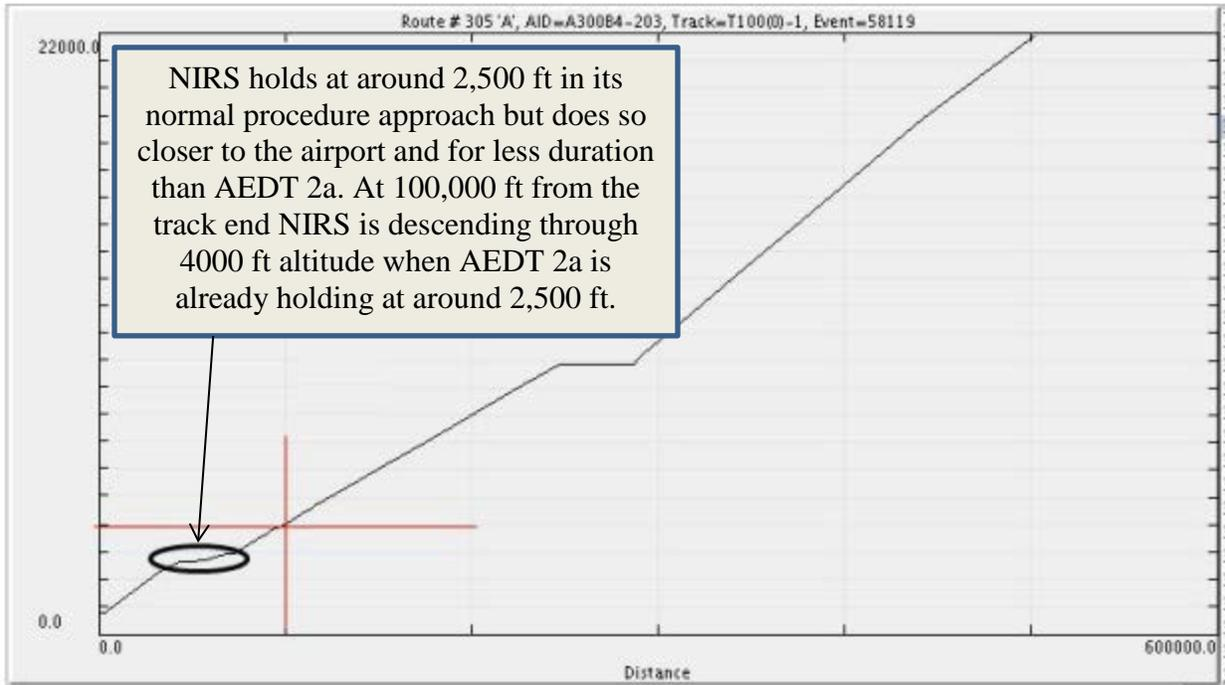
Figure 4-13: NIRS Arrival Profile for A300B4-203 on track T100
